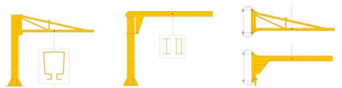
Gru a bandiera a colonna e mensola in rotazione manuale / Column-mounted and bracket mounted jib cranes with manual rotation
